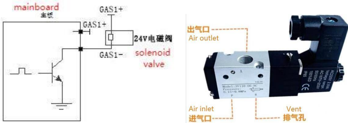
Figure 2.121 Schematic diagram of the gas control interface
