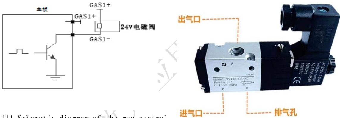
Figure 2.111 Schematic diagram of the gas control interface
