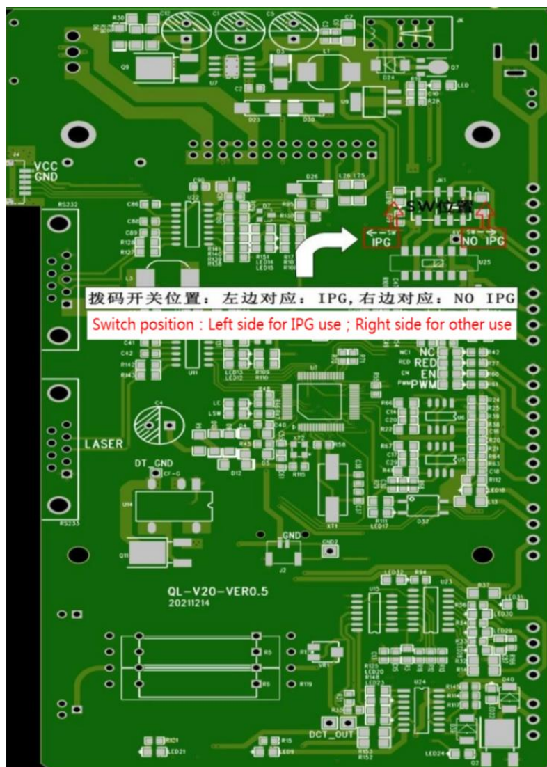
Figure 2.13, schematic diagram of dial switch
