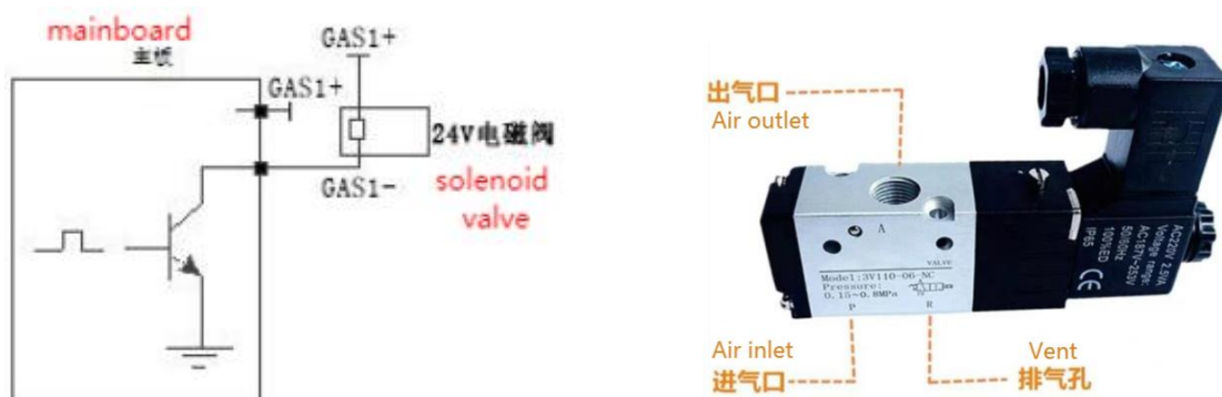
Figure 2.121 Schematic diagram of the gas control interface
