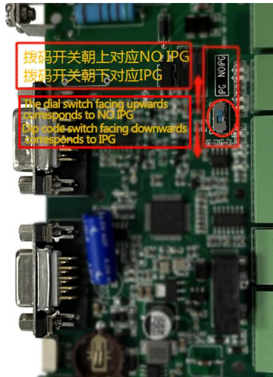
Figure 2.15, schematic diagram of dial switch
