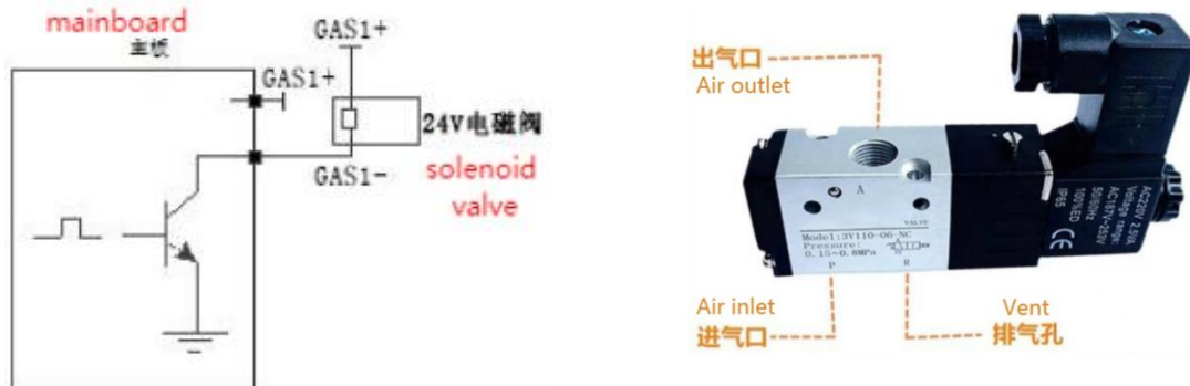
Figure 2.11.1, a schematic diagram of the gas control interface
