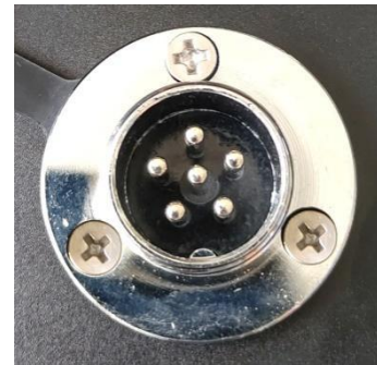
Connecting port of wire feeder control box
